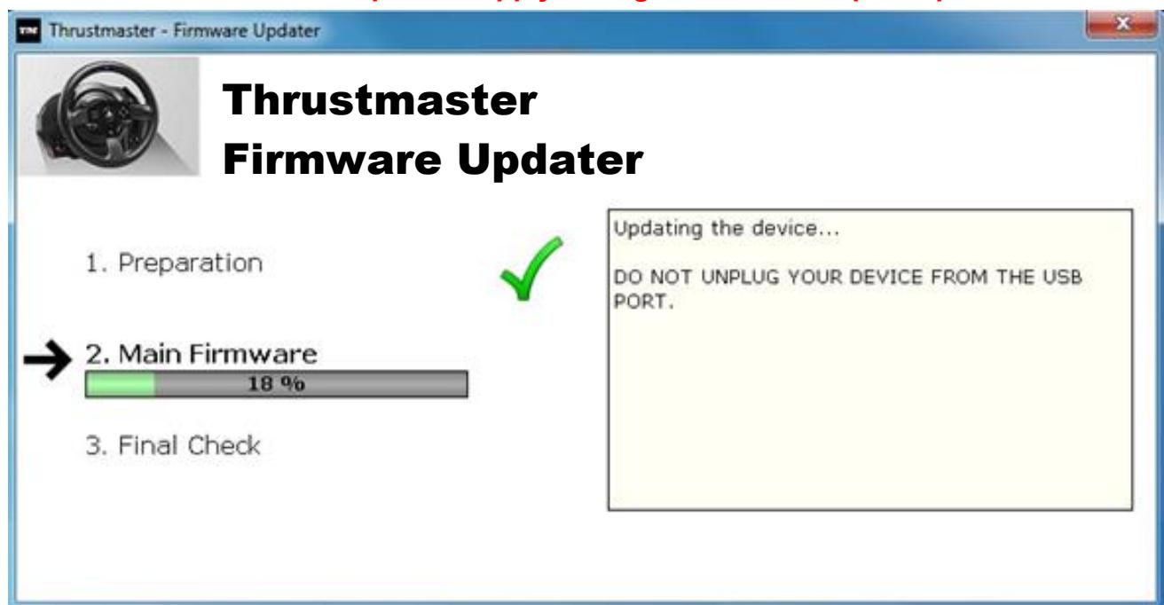
The firmware update procedure begins (the update progress is displayed onscreen). During the firmware update, the **MODE** LED on the wheel will be OFF: this is perfectly normal.
